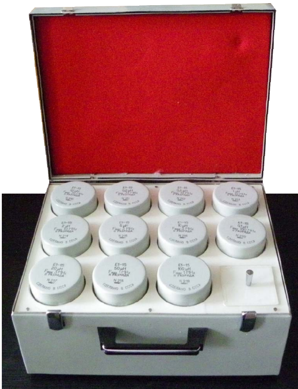
Fig. 1. Pictorial view of the standards E1-15.
