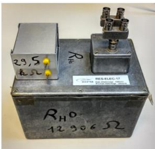
Figure 3.1.5: Enclosure containing the Vishay resistor, with a 4-terminal-pair adaptor and the thermistor pins.
