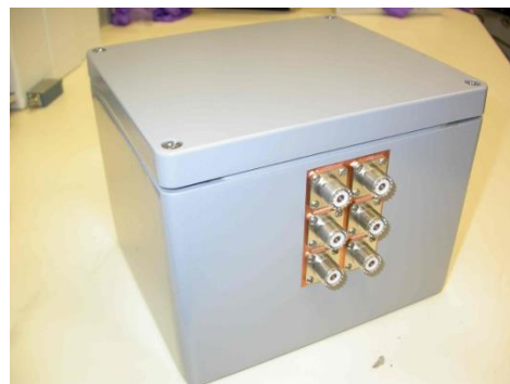
Figure 3.1.2: Temperature-controlled enclosure containing the hermetic brass enclosure
