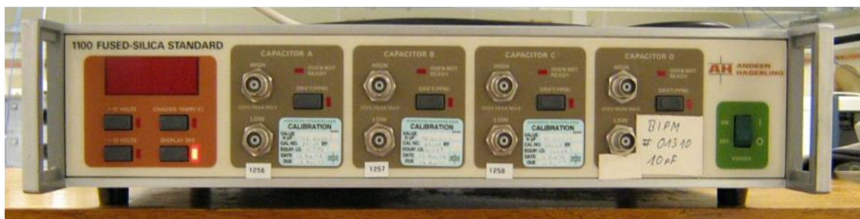
Figure 4.1: The travelling Andeen-Hagerling frame with four capacitance standards.
