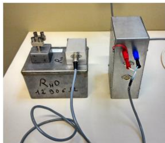
Figure 3.1.6: Vishay resistor and power supply of the temperature controller.
