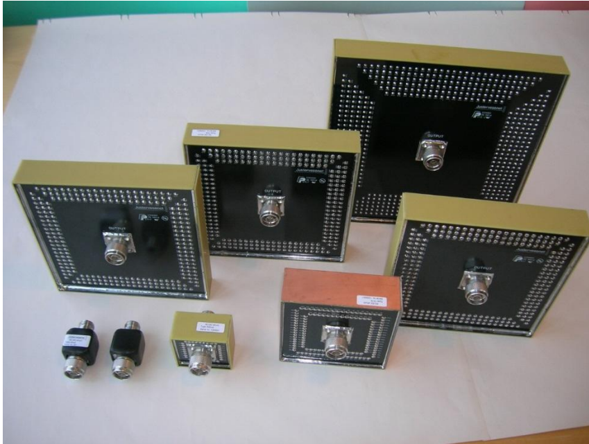
Figure 1: The current shunts viewed from the output side. The 20 A shunt has UHF input connector, while all the others have N connectors.
