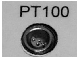
Fig. 3b. LEMO connector for the internal PT100 thermoresistance
