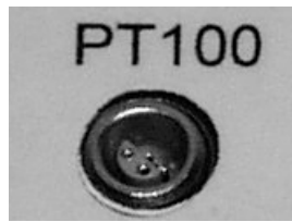
Fig. 3. LEMO connector for the internal PT100 thermoresistance
