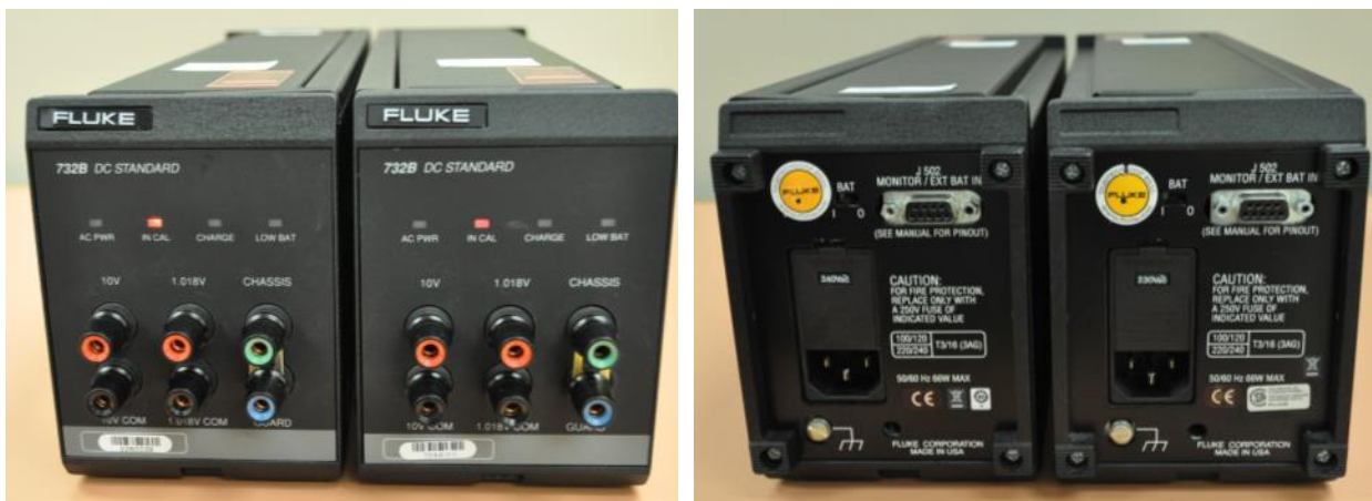
Figure 1 Photos showing front view and rear view of a Fluke 732B
