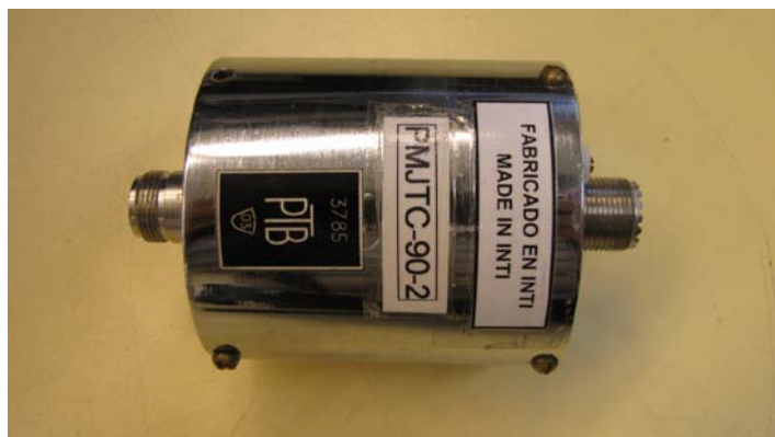
Fig.1. Physical layout of the thermal converter PMJTC-90-2
