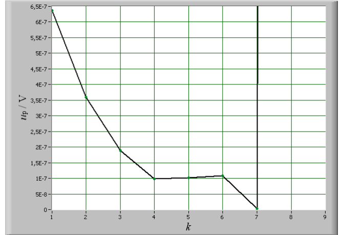
Fig. 4. Distribution of calculated uncertainties u_p of DCRS-RU at the 1,018-volt level (the index k shows which data are rejected in the analysis, and corresponds to the no. in Table II).
