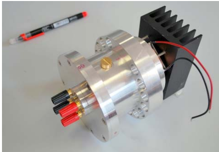
Fig. 1. Aluminium box. The block connected with a TEC and a radiator is shown.
