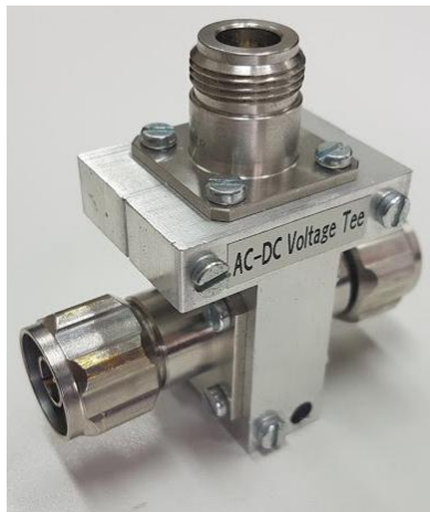
Figure 11.9: AC-DC Voltage Tee used in difference comparator system.
