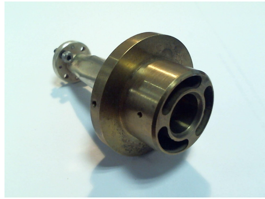
Figure 2.2: Front view of waveguide taper showing central hole for location of the waveguide tube and three slots in the brass supporting ring to carry the low frequency coaxial cables.
