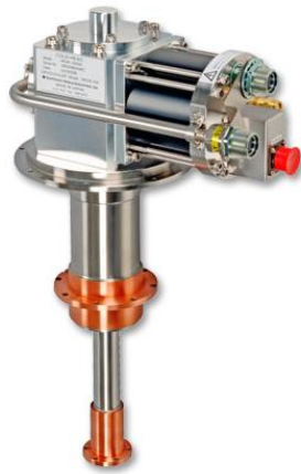
Figure 5.4: Typical 1 W at 4 K commercial Gifford-McMahon (two stages) cryocoolers [44]. The typical intermediate stage temperatures are around 30 K to 35 K (with no thermal charge). It can provide about 40 W at 45 K.
