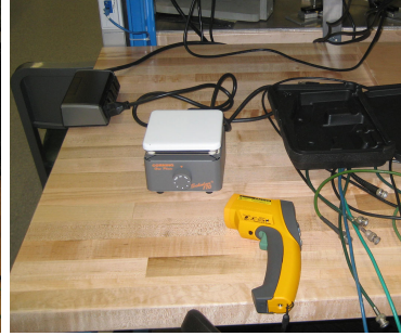
Figure 7: Hot Plate for heating points and IR Temperature meter Click here to see larger picture
