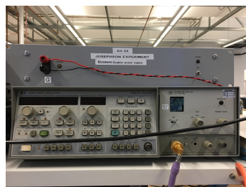
Figure 3: Power Supply, Sweep Oscillator, and RF Plug-in Click here to see larger picture
