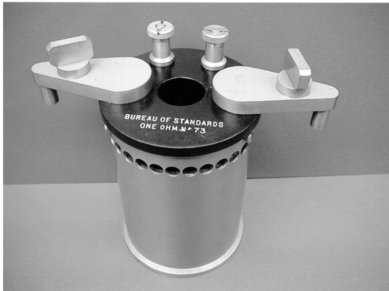
Fig. 1. A double-walled 1 \Omega standard resistor of the Thomas type.
