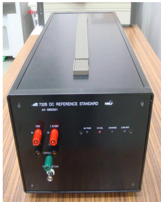
Fig. 1: An upgrade-box with Fluke 732B and additional batteries (inside).
