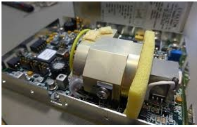
Fig. 49. Datum LPRO RFS. Photo Credits: Datum.
