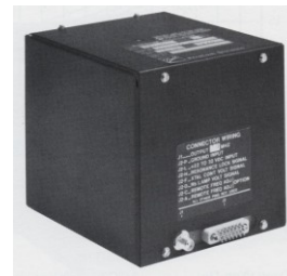
Fig. 47. Efratom FRK Commercial RFS. Quoting from the Smithsonian National Museum of American History web site for this item: “This compact rubidium frequency standard is the commercial Model FRK, first made by Efratom Elektronik, Munich, Germany, and later by Efratom California in Irvine, Ca. Gerhard Hübner and Ernst Jechart established the firm in 1971 and a year later supplied examples of the clock to the Naval Research Laboratory (NRL), Washington, D.C., for inclusion on NTS-1, the first of the Navigation Technology Satellites (NTS) launched in 1974 to validate the key concepts and hardware for the Global Positioning System (GPS). Relatively large rubidium frequency standards had been developed in the 1950s, but the FRK—weighing roughly three pounds and measuring about four inches on a side—were the smallest atomic frequency standard of any type available. Efratom established a branch in Irvine, California, in 1973 and manufactured compact rubidium frequency standards there for a variety of customers. The firm became a division of Ball Aerospace in 1982 and then part of Datum in 1995. Symmetricom acquired Datum in 2002.” Photo Credit: Ball Efratom (More photos on the Smithsonian web site ).
