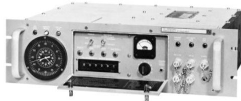
Fig. 29. Collins Radio AFS-81 Military RFS. The AFS-81 contained an Rb physics package made by General Radio. Photo Credit: Collins Radio.
