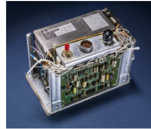
Fig. 33. Rockwell GPS RFS. This atomic clock was built for the first GPS satellites in the late 1970s [119]. Photo Credit: Smithsonian Museum.
