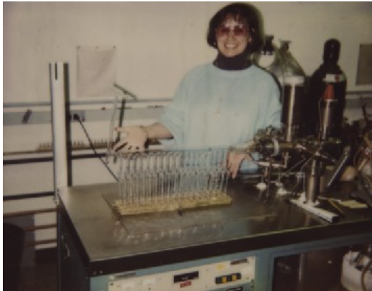
Fig. 11. Rb Lamp Processing. A manifold of Rb lamps attached to a high vacuum processing system. Photo Credit: EG&G.
