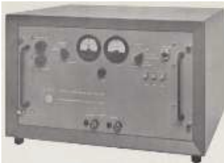
Fig. 19. Varian V-4700A. The 1 st commercial rubidium frequency standard. Photo Credit: Varian Associates
