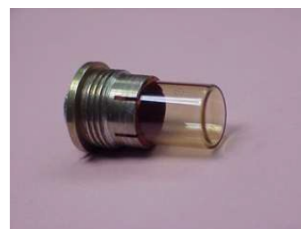
Fig. 9. Rb Lamp. This is a GPS RAFS lamp in its screw-in holder. Photo Credit: PerkinElmer.
