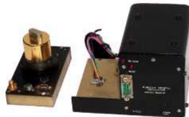
Fig. 45. EG&G RbXO with TMXO (left). Photo Credit: EG&G.
