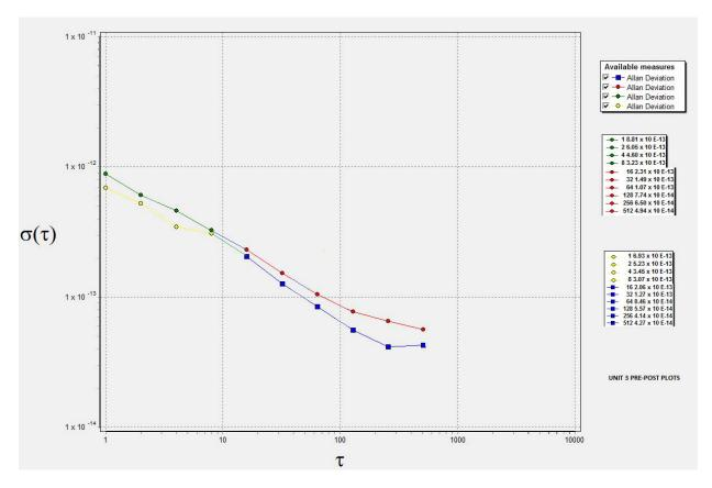
Unit three had amazing pre-mod performance! It was better that any unit I have ever seen! A "good" performing 5065A normally is comparable to the pre-mod plots of the prototype and units 1 & 2. (This is out of a sample of over 50 5065A units.)
