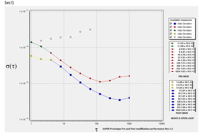
This plot shows the pre-mod versus the post-mod stability of the prototype unit as well as the free running or open loop stability of its 10811 Quartz oscillator. The Prototype was evaluated against an Active Maser here, an Active Maser at Tom Van Baak's, and a Passive Maser at another site.
