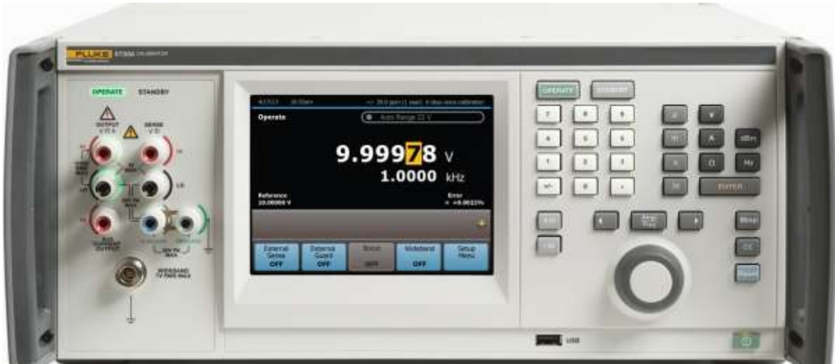
Figure 2. Keithley uses a Fluke 5730A Multifunction calibrator to calibrate multimeters. Photo courtesy of Fluke.
