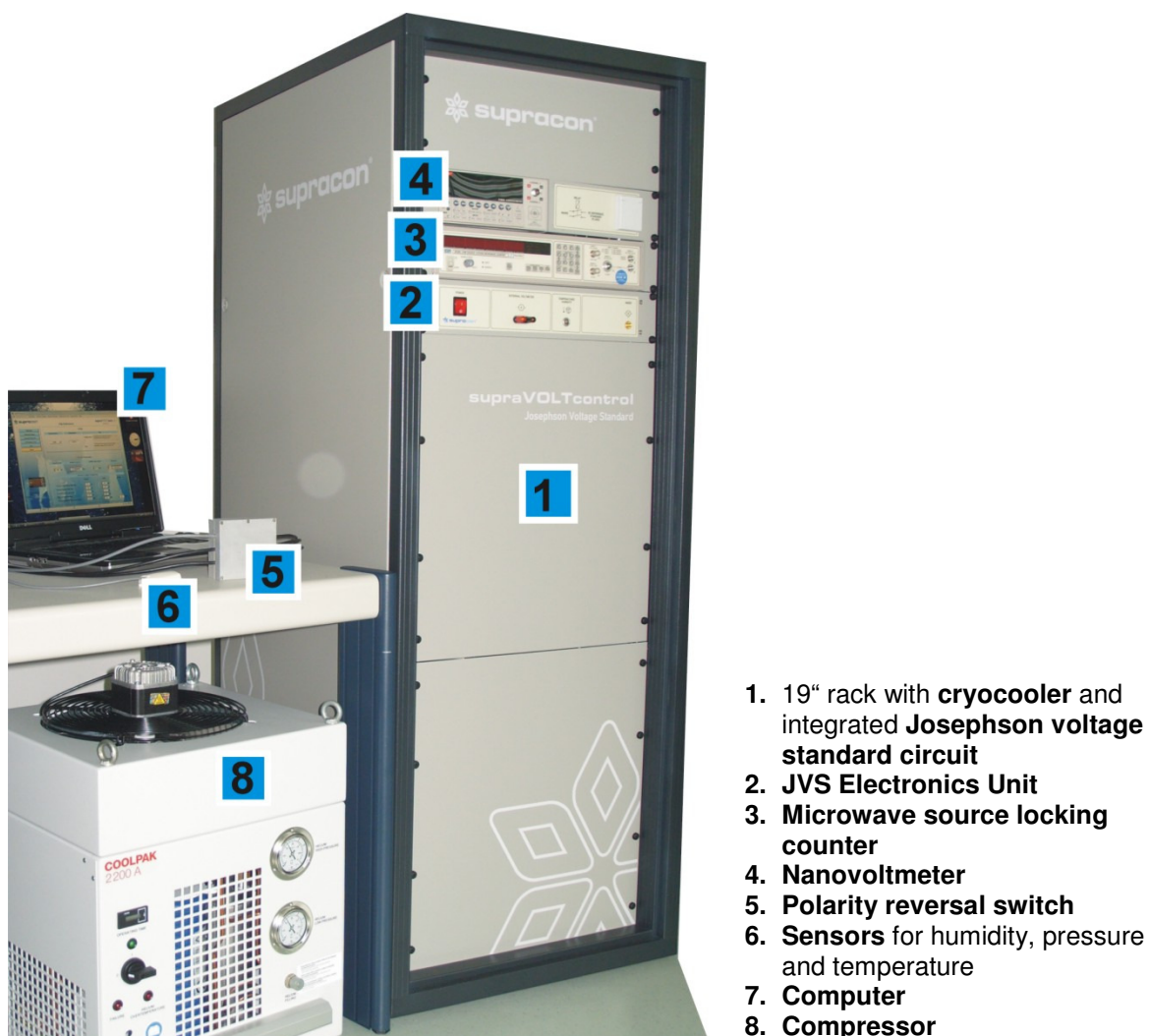
Figure 15: Cryocooler-based Josephson voltage standard system "SupraVOLTcontrol".
