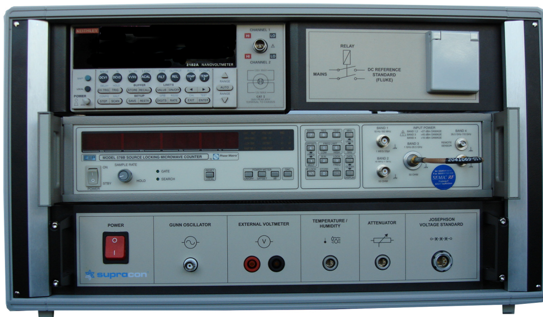
Figure 8: Front panel of the JVS electronics unit installed at the bottom of the 19" rack (liquid helium version).
