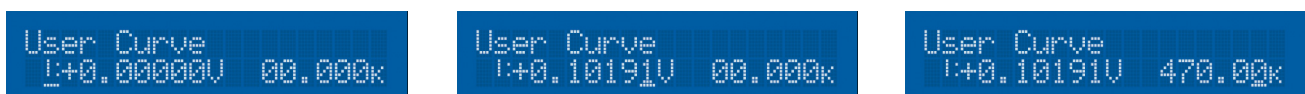
FIGURE 5-8 Left: Scroll to highlight a breakpoint number; Middle: Press the enter key to highlight the sensor value of the selected pair ; Right: Press the enter key again, and the temperature value is highlighted
