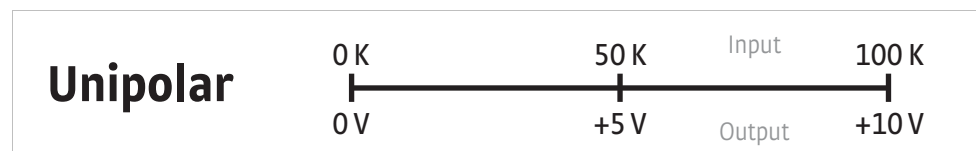
FIGURE 5-5 Output with polarity parameter set to unipolar
