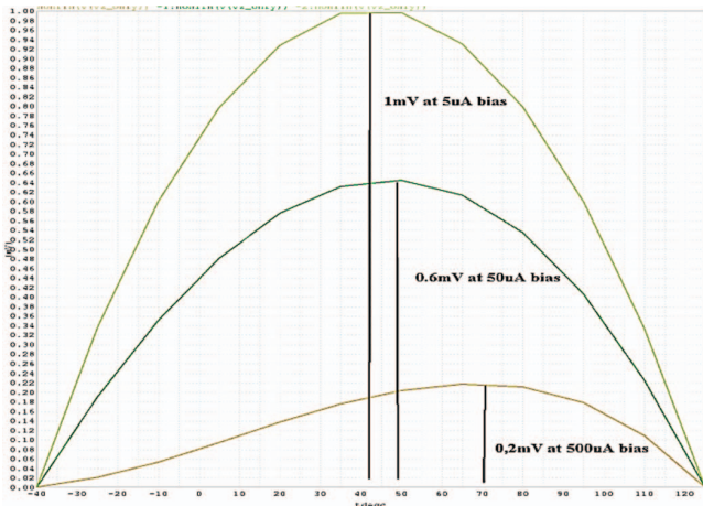
Fig. 7. Temperature nonlinearity dependency at different bias currents
