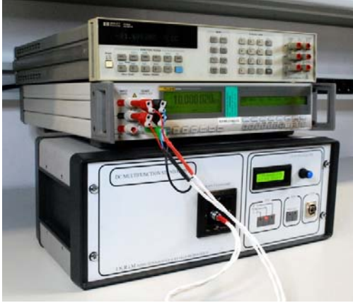
Fig. 2. View of the RSU calibrating high precision DMMs. The selected standard is available at a LEMO four-pole connector whose shield is connected to the guard and to the temperature control minimizing the temperature difference between it and the connectors of a connected instrument lowering the emfs.
