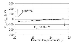
Fig. 6. Voltage error ( $V_{OUT}$ - $V_{SET}$ ) at the output of the circuit in Fig. 5 versus external temperature. The temperature control system is active in the range from 22.2 to 24.8 °C. Outside this range the temperature control circuit is saturated and therefore the temperature coefficient of the voltage source is -2N mV/°C.
