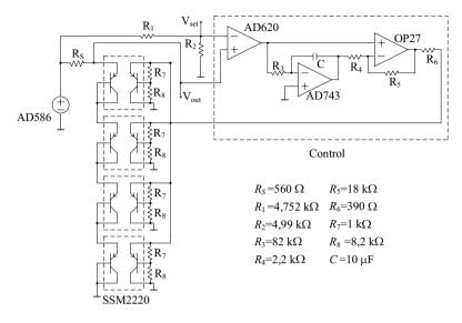
Fig. 5. Complete schematic of the low noise voltage reference including the temperature compensation system. The circuit within the dashed box acts as an error amplifier with a proportional-integral action. By changing the current supplied to the transistors used as heaters, the voltage  $V_{OUT}$  is made to approach the target voltage  $V_{SET}$ .
