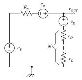
Fig. 3. Small signal equivalent circuit for the calculation of the output voltage noise. The equivalent noise source  $e_D$  accounts for the noise introduced by the N diodes as discussed in the text.
