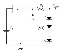
Fig. 1. A simple implementation of a low noise voltage reference. The number N of diodes connected in series together with the values of  $R_s$  and of the reference voltage  $V_R$  set the output voltage.
