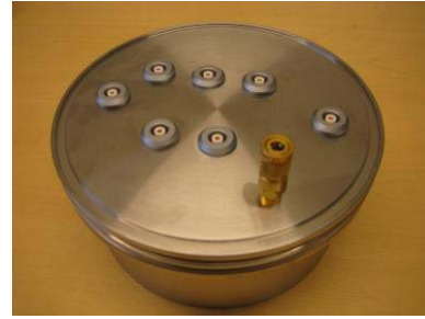
Fig. 3. Low-voltage arm in a sealed container filled with SF 6 .
