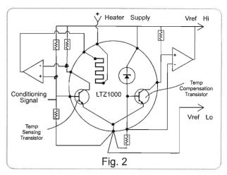
control loop. This leaves the sensing transistor free to be used as an <u>independent</u> temperature monitor.
