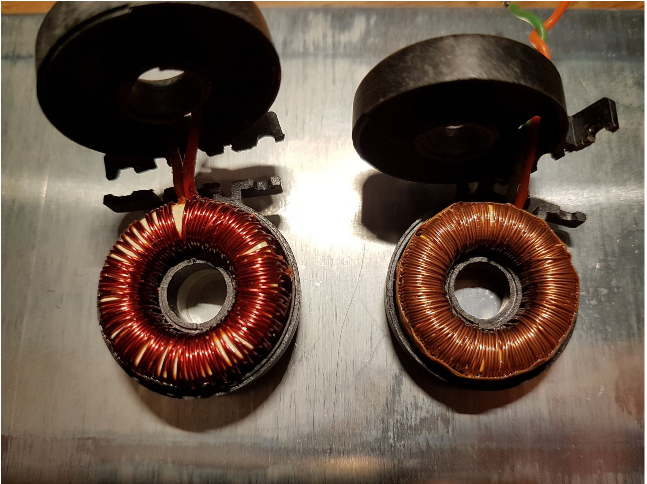
Figure 6: Wavetek & early Fluke 7000 transformer of DC-DC converter – primary side (left), secondary side (right)
