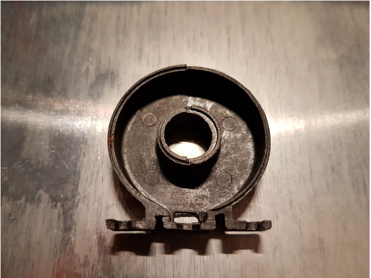
Figure 9: Wavetek & early Fluke 7000 transformer of DC-DC converter – single screen component
