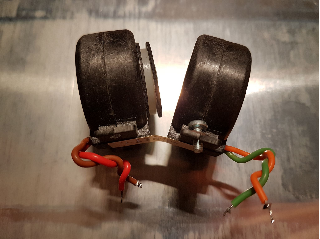
Figure 5: Wavetek & early /Fluke 7000 transformer of DC-DC converter – coupling winding removed
