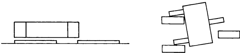
Figure 9.1 Open joints caused by: (a) lack of coplanarity; (b) wicking
