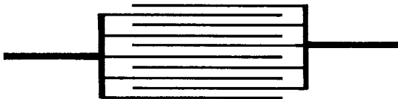
Figure 8.20 Comb pattern for a SIR test
