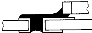
Figure 6.11 Footprint starved of solder by neighbouring via. Remedy: a bridge of solder resist between the via and the component footprint
