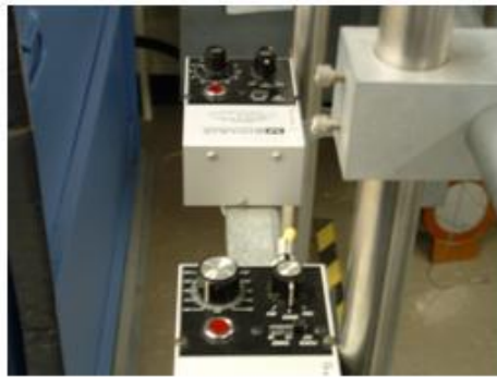
Chamber alignment controls 100 kV range
