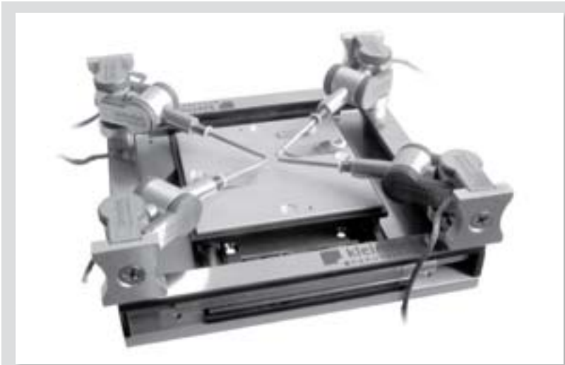
Figure 2. Example of a powerful, dedicated system for electrical characterization of nano and semiconductor devices and advanced materials. (Graphic courtesy of Kleindiek Nanotechnik.)
