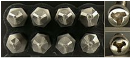
First row: Tri-Wing bits and screw head. Beneath: Tri-Point/Y-Type.
