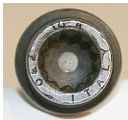
End view of M10 triple square screw
