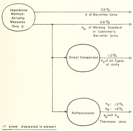
$$\eta = \frac{\text{rf power dissipated in element}}{\text{rf power dissipated in unit}}$$
