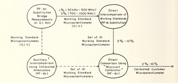
Each Set of 10 Working Standards is Intercompared by Two Different Techniques as an Internal Check.
