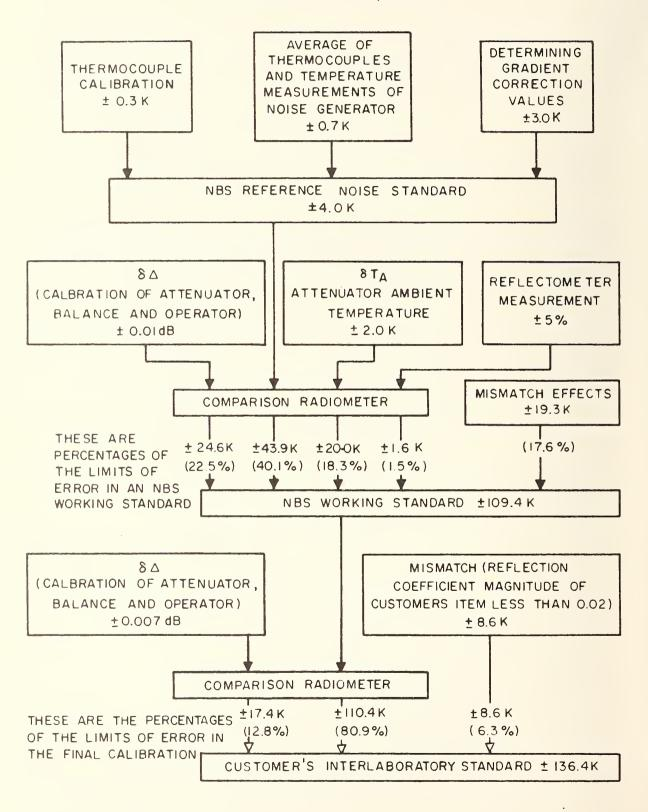
Effective Noise Temperature For Argon Noise Source, or Waveguide Noise Source at 9 GHz 11,000 K
