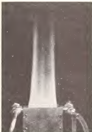
FIG. 2. Photograph of flame on slot burner. The reaction zone is the small bright line just above the burner. The remainder of the luminous zone is due to the hot gases in which there is little chemical reaction.
