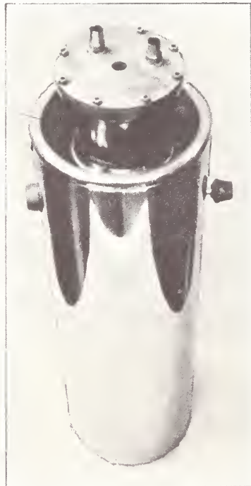
Fig. 3—Assembled vacuum deposited outer conductor line with cryostat.
