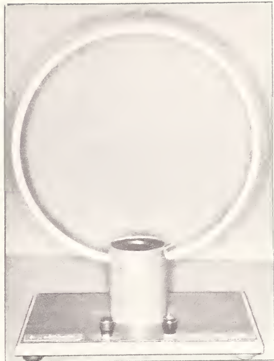
Fig. 4 - A 10 MHz Standard Receiving Loop Antenna
