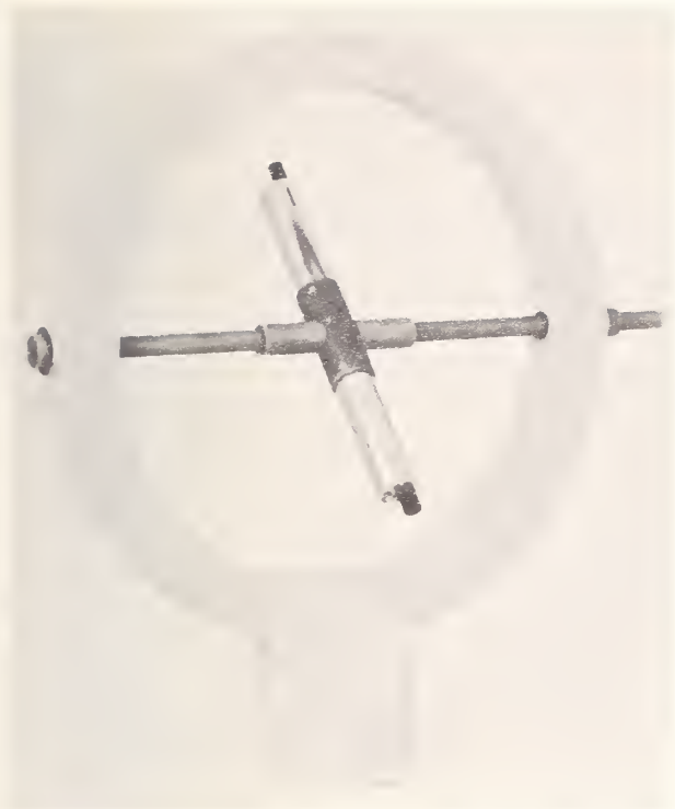
FIGURE 4. View of the measuring dipole and mounting gimbal.
