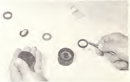
Fig. 1—An RF permittimeter with standard ring, shorting ring and various rings of materials to be measured.
