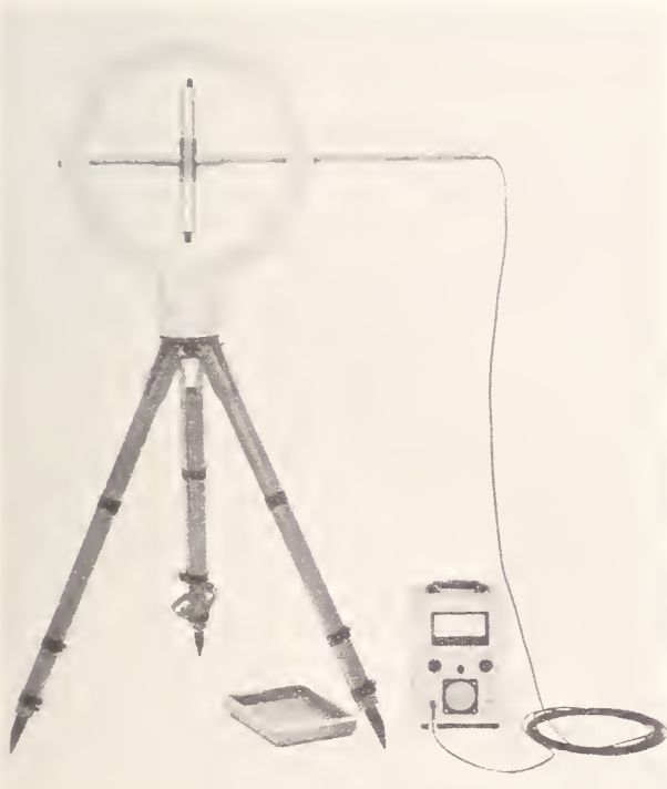
FIGURE 5. The complete near-zone field-strength meter.
