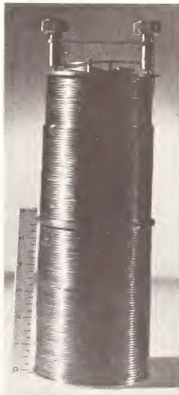
Fig. 2—Two \mu\text{sec} heavy lead FEP Teflon line.
