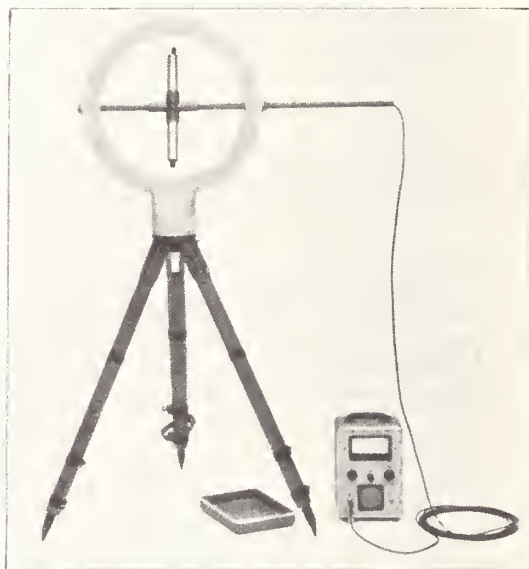
Fig. 14. View of the complete near-zone electric-field-strength meter.
