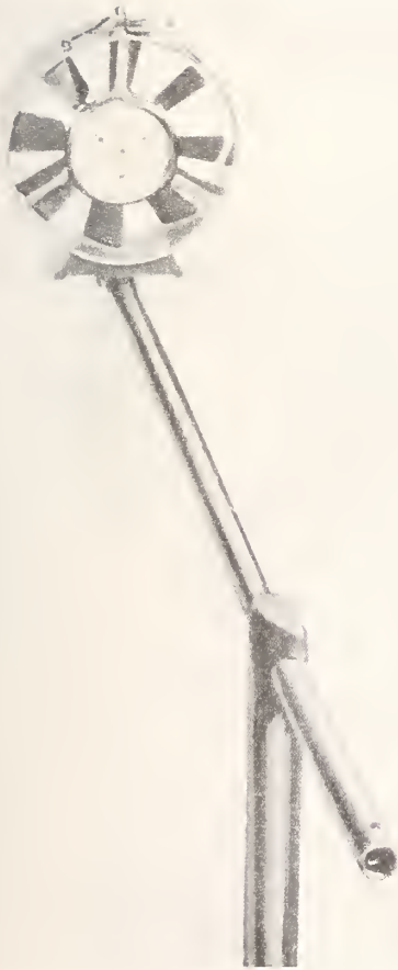
FIGURE 2. Anemometer supported on rod.
