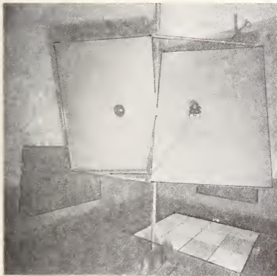
FIG. 1. View showing vanes in the reverberation room of the National Bureau of Standards.
