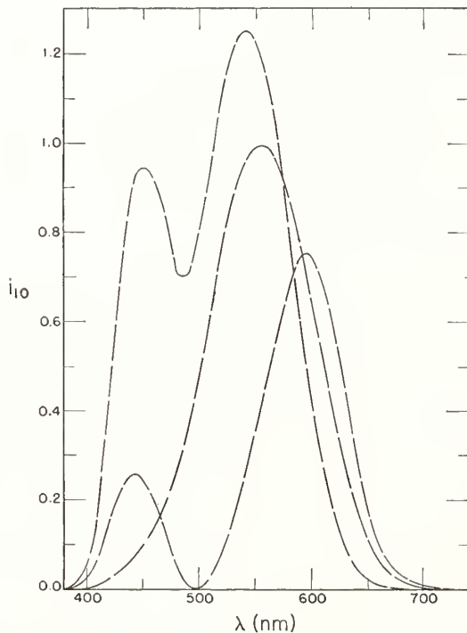
FIG. 3. Spectral tristimulus values i_{10} for the 10^\circ observer system. The spectral tristimulus values and the chromaticity
