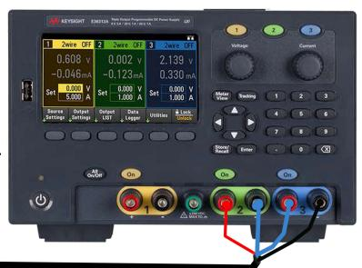
Option C: PSU with two non-isolated channels Linear lab power supply with two channels capable to provide +12V each at 100mA will work good here. Such example is Keysight E3631A PSU. Connect +12V lead to CH2 HI and -12V lead to NEGATIVE CH2 RED post. Both blue FX GND connect to COM. Set curent limit 0.1A for +12/-12V outputs.
