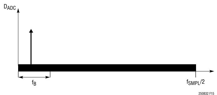
Figure 15. Frequency Spectrum of SAR ADC Core Output
