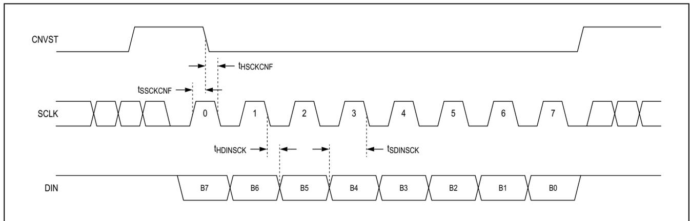
Figure 4. Input Configuration Timing in CS Mode
