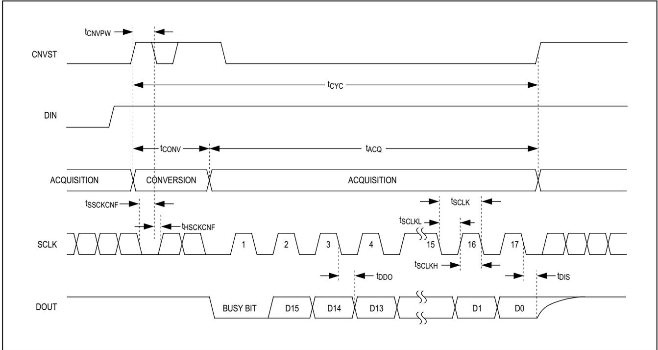
Figure 9. CS With Busy Indicator Mode Timing
