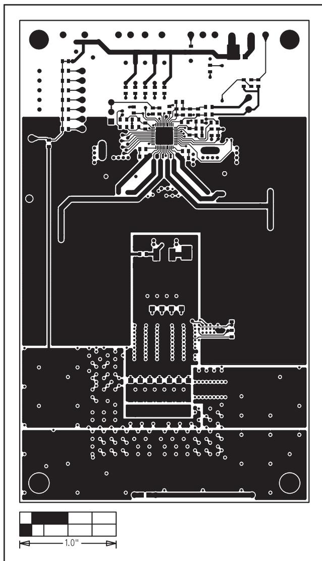
Figure 10. MAX17582 EV Kit PCB Layout—Solder Side
