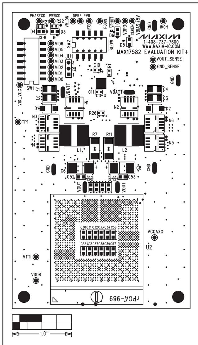
Figure 2. MAX17582 EV Kit Component Placement Guide—Component Side
