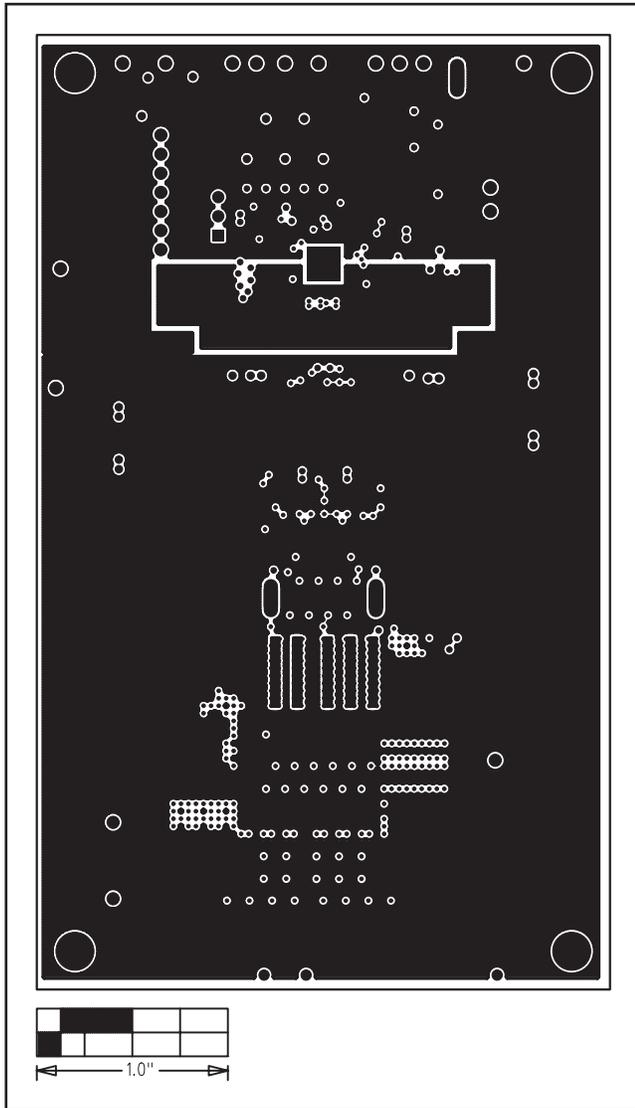
Figure 4. MAX17582 EV Kit PCB Layout—Internal Layer 2 (VBATT/PGND Plane)
