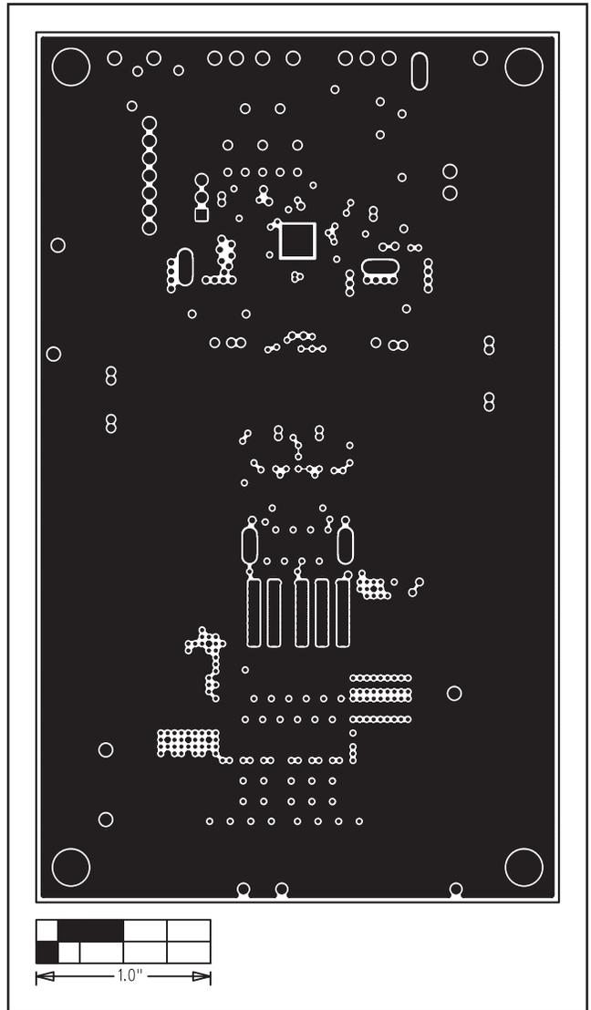
Figure 9. MAX17582 EV Kit PCB Layout—Internal Layer 7 (PGND Layer)
