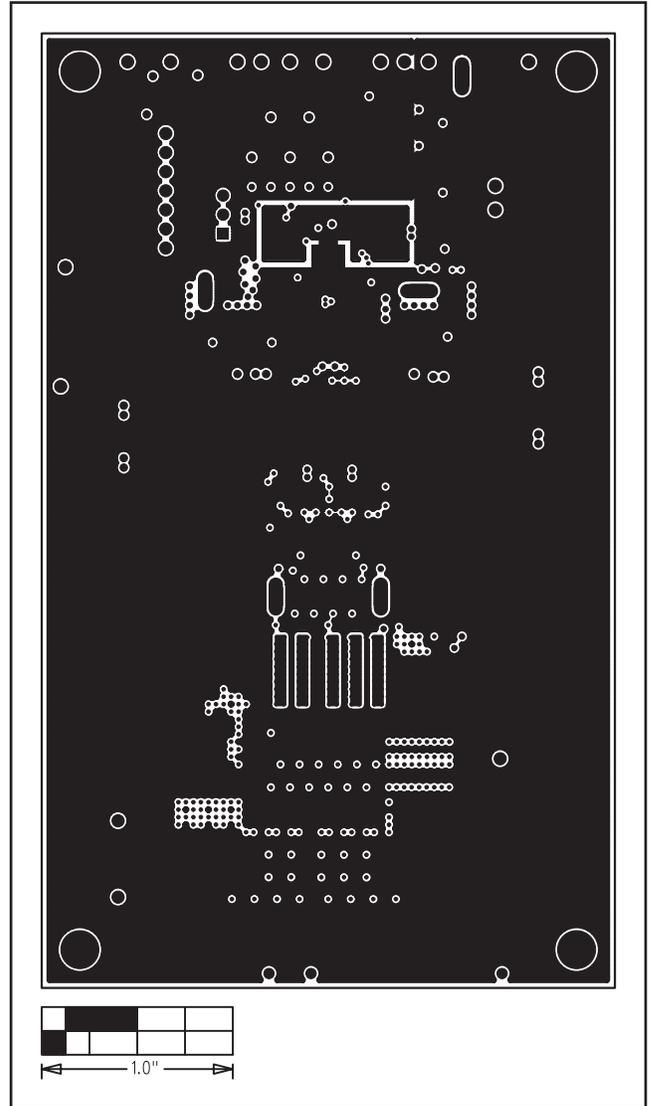
Figure 7. MAX17582 EV Kit PCB Layout—Internal Layer 5 (AGND/PGND Layer)
