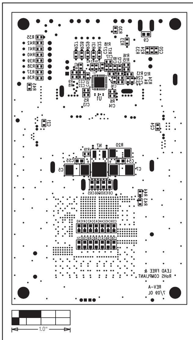
Figure 11. MAX17582 EV Kit Component Placement Guide—Solder Side
