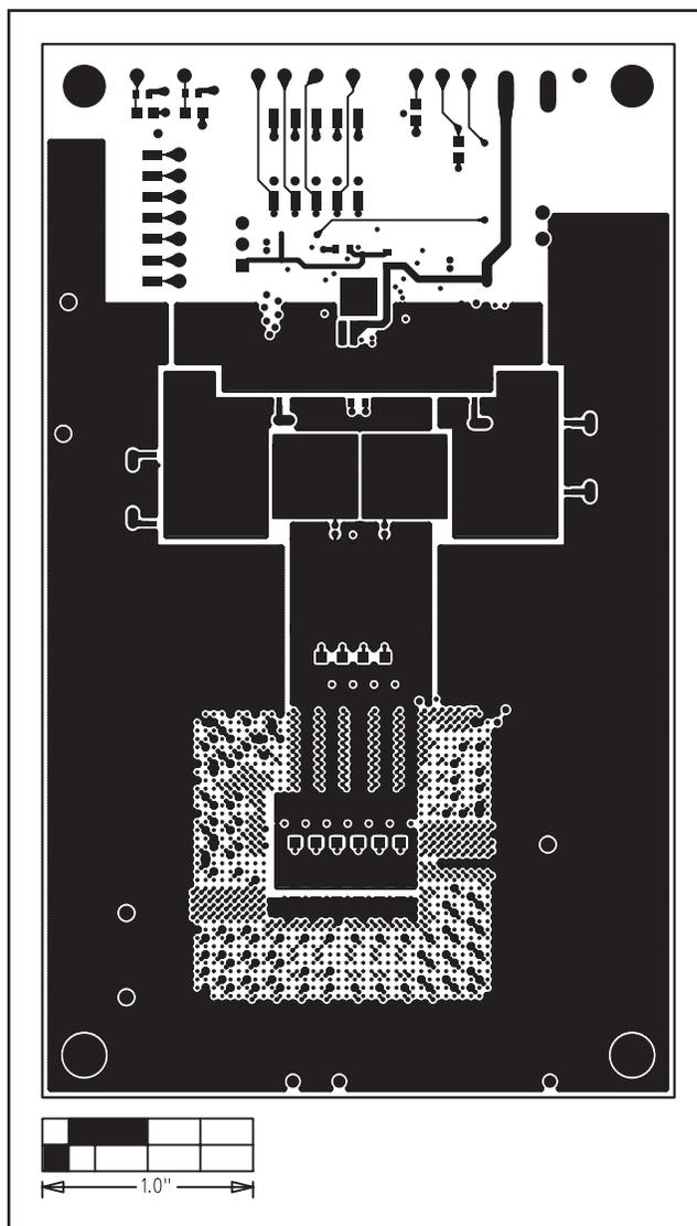
Figure 3. MAX17582 EV Kit PCB Layout—Component Side
