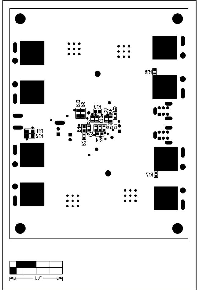
Figure 5. MAX5944 EV Kit Component Placement Guide—Solder Side
