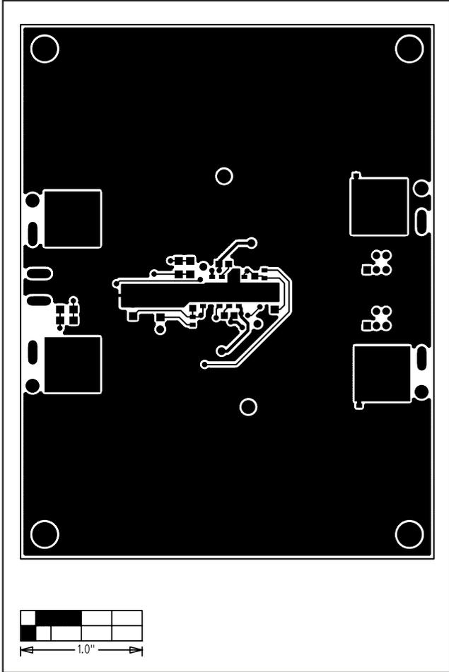
Figure 4. MAX5944 EV Kit PC Board Layout—Solder Side
