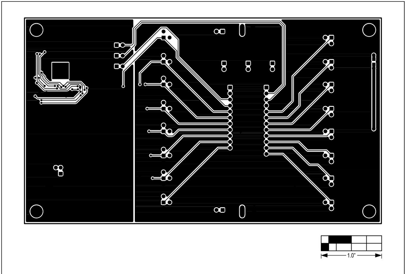
Figure 6. MAX7358 EV Kit PCB Layout—Solder Side
