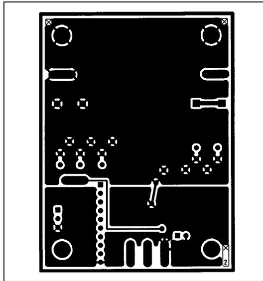
Figure 4. MAX849 EV Kit PC Board Layout—Solder Side
