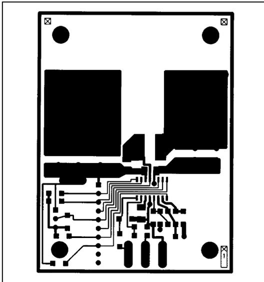
Figure 3. MAX849 EV Kit PC Board Layout—Component Side
