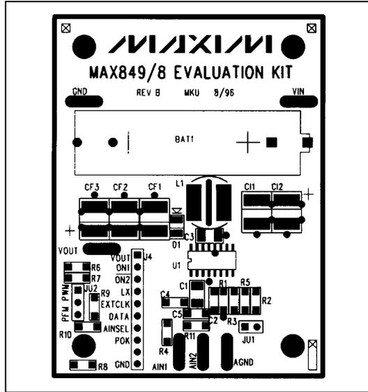
Figure 2. MAX849 EV Kit Component Placement Guide
