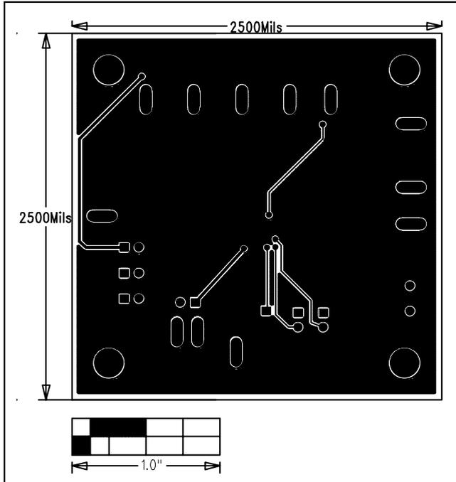
Figure 6. MAX8677A EV Kit PCB Layout—Layer 3
