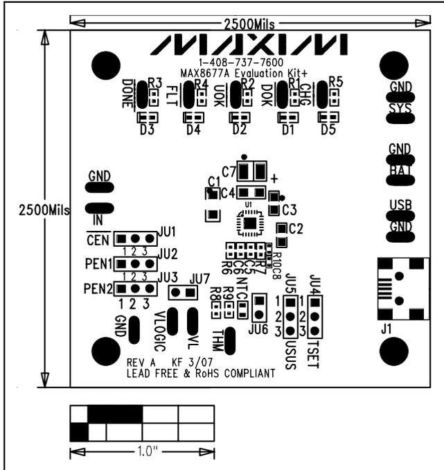
Figure 3. MAX8677A EV Kit Component Placement Guide—Component Side
