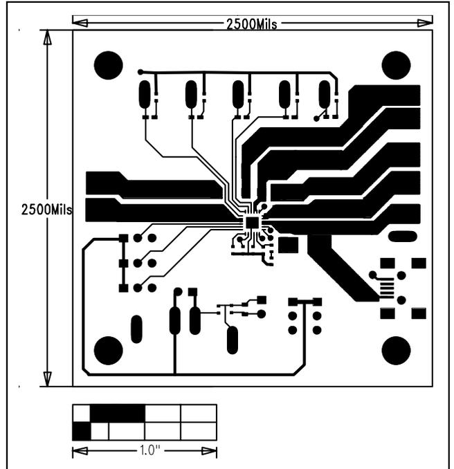
Figure 4. MAX8677A EV Kit PCB Layout—Component Side
