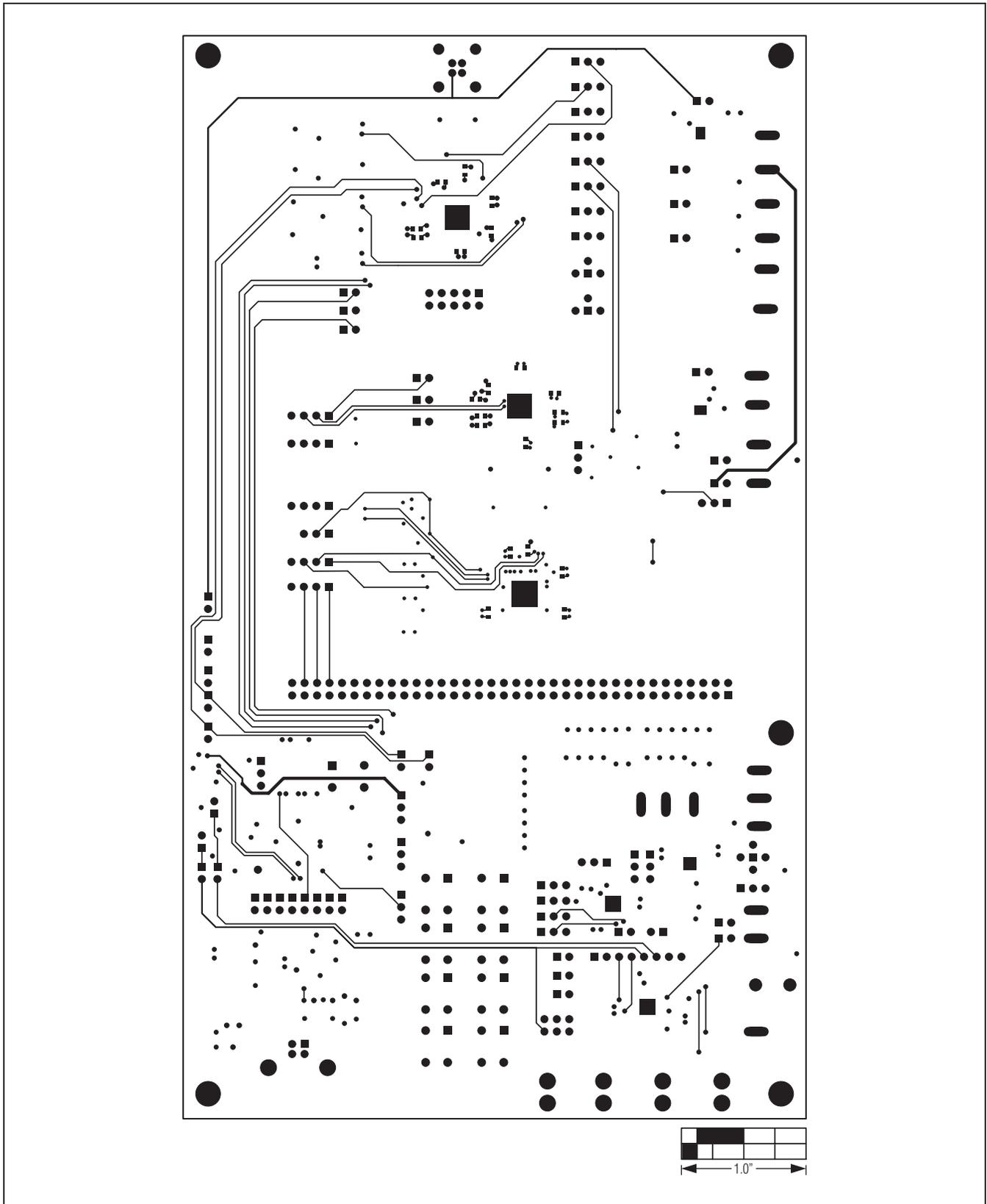
Figure 15. MAX9266 EV Kit PCB Layout—Solder Side
