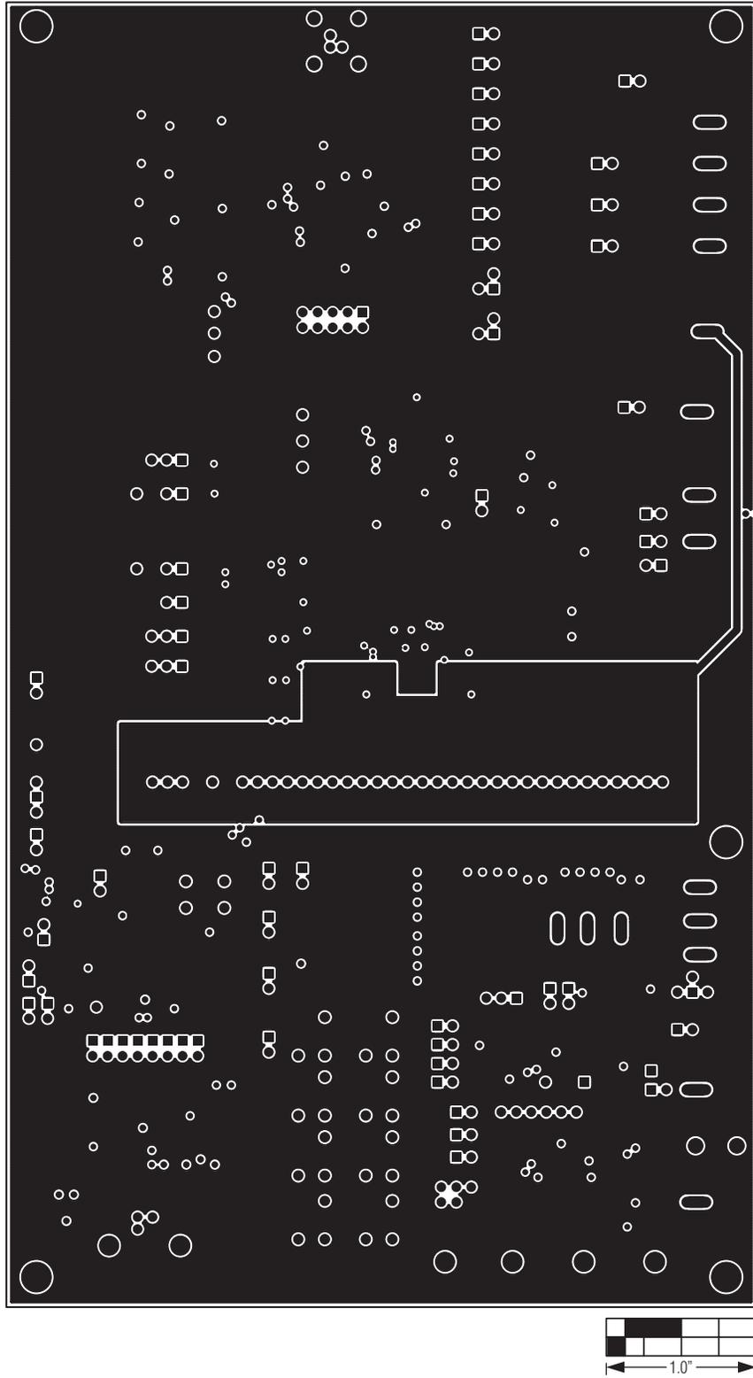
Figure 13. MAX9266 EV Kit PCB Layout—Ground Layer 2
