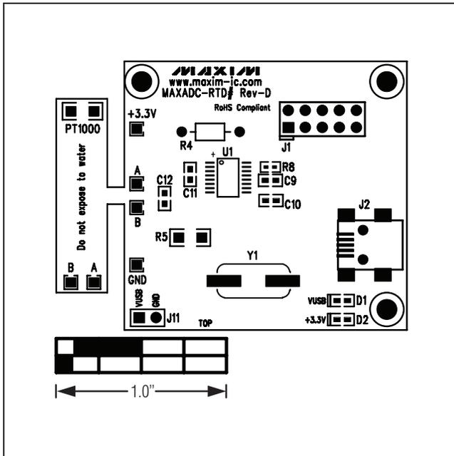
Figure 4. MAXADC-RTD Component Placement Guide—Component Side
