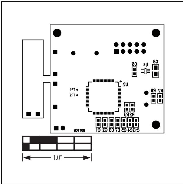
Figure 5. MAXADC-RTD Component Placement Guide—Solder Side
