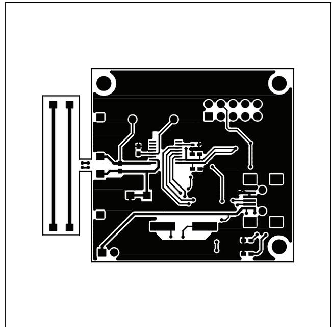
Figure 6. MAXADC-RTD PCB Layout—Component Side
