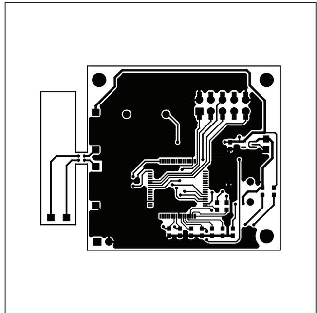
Figure 7. MAXADC-RTD PCB Layout—Solder Side
