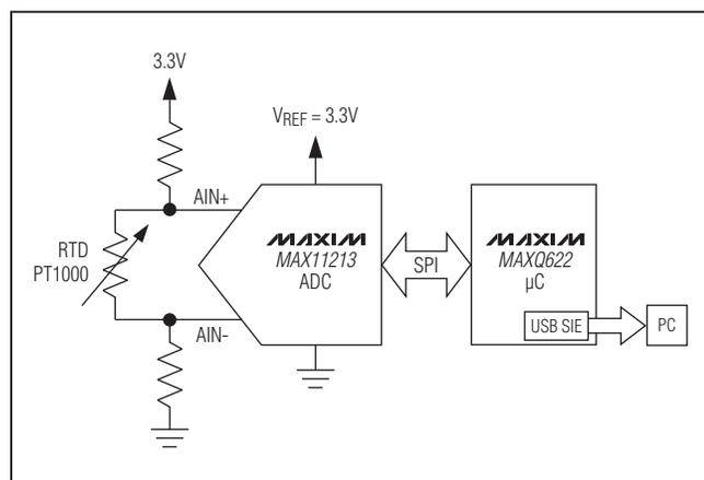
Figure 1. MAXADC-RTD Block Diagram
