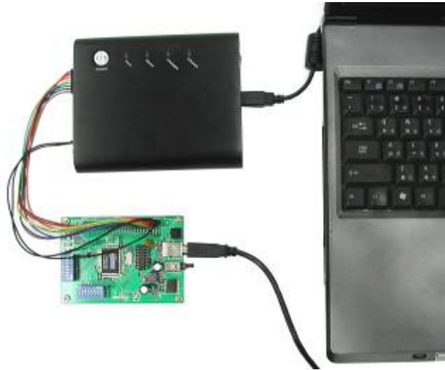
Fig. 2-6: An Assembly of Laptop, Logic Analyzer, and Testing Board
