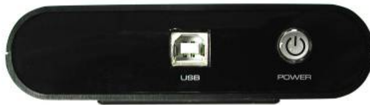
Fig. 1-10: Side view of AKIP Logic Analyzer, which draws its power from the USB connection.
