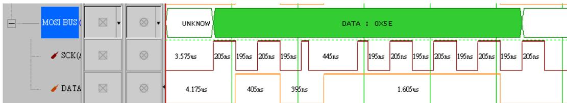
3. Clock Phase (CPHA) = 1 , Clock Polarity (CPOL) = 0 :
