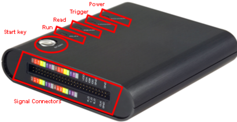
Fig. 1-9: A View of the AKIP Logic Analyzer. See Fig 1-11 for detailed information on the Signal Connectors .
