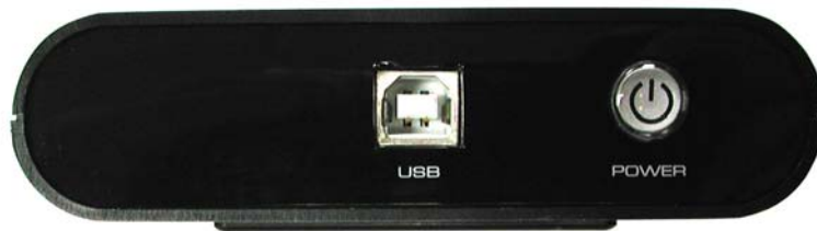
Fig. 1-10: Side View of the AKIP Logic Analyzer; the power of the Logic Analyzer is drawn from the USB connection.
