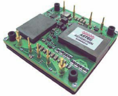
(b) 400 W Half-brick DC-DC Converter Ref. [2.32]
