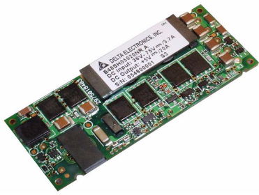
(a) 120 W Eighth-brick DC-DC Converter Ref. [2.31]
