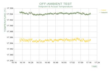
Once converted, calculate the error signal between actual and setpoint temperatures.
