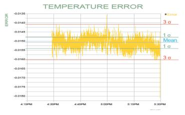
Determine the approximate time from the X-axis that this point occurs. This point is the origin marker in the data set for computing the temperature stability. For 1-hour stability, ensure that the data set duration is at least 1 hour. For 24-hour stability, ensure that the data set duration is at least 24 hours.
