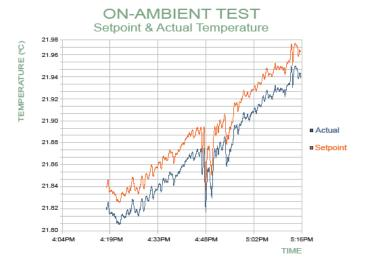
Again, the controller and load are not in a temperature controlled chamber. They are out on a test bench experiencing ambient fluctuations with air conditioning and heating changes. These specifications are deliberately measured this way to show robustness.
