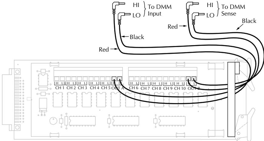
**Note:** OUT B connections not required for 2-pole operation. Plastic shield not shown.
