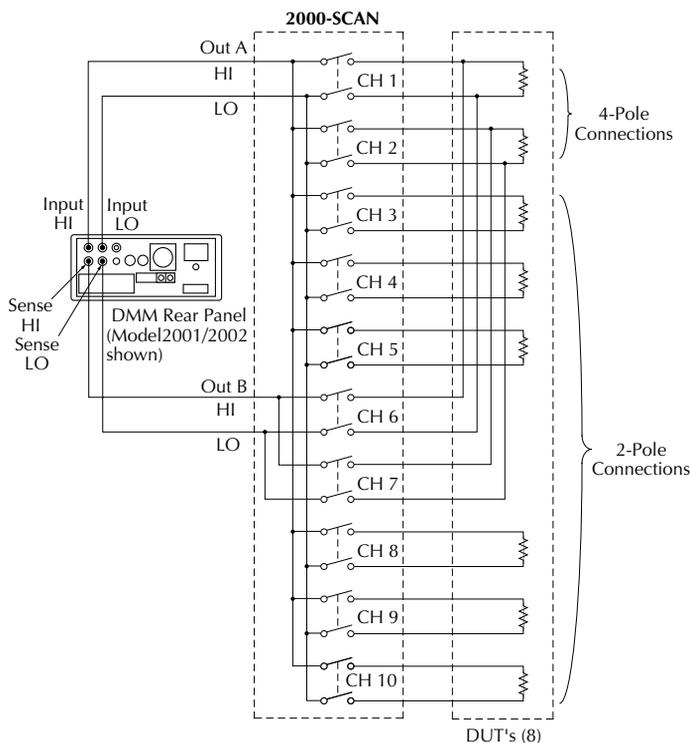
Measurement functions for each scanner channel are defined using the INTERNAL-CHANS menu available by pressing CONFIG-CHAN (see [“Using the scanner with the buffer” on page 3–13](#)). Measurement functions for this test would be set up as follows:
