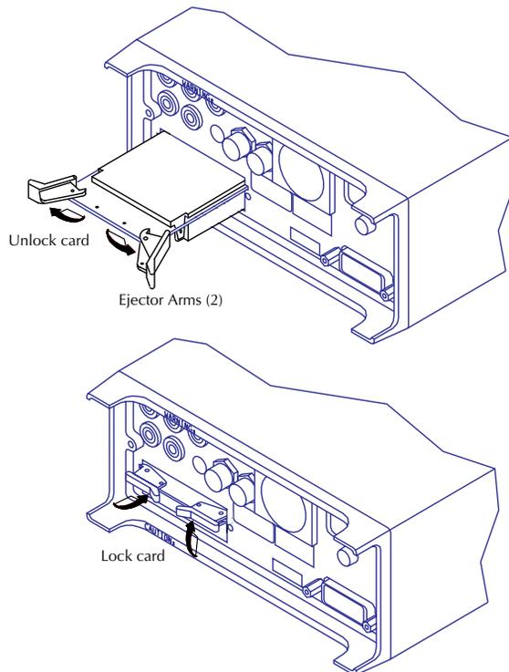
Note: Card installation in a Model 2001/2002 is shown. For installation in Model 2000, turn card over.
