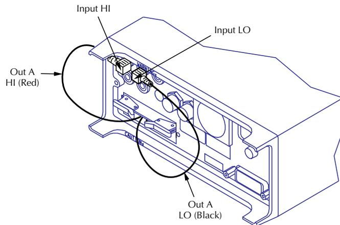
Note: Card installation in a Model 2001/2002 is shown. For installation in Model 2000, turn card over.
