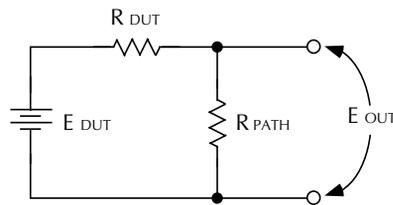
$$E_{OUT} = \frac{E_{DUT} R_{PATH}}{R_{DUT} + R_{PATH}}$$
