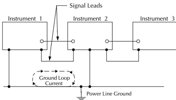
[Figure 3-8](#) shows how to connect several instruments together to eliminate this type of ground loop problem. Here, only one instrument is connected to power line ground. Ground loops are not normally a problem with instruments having isolated LO terminals. However, all instruments in the test setup may not be de-signed in this manner. When in doubt, consult the manual for all instrumentation in the test setup.
