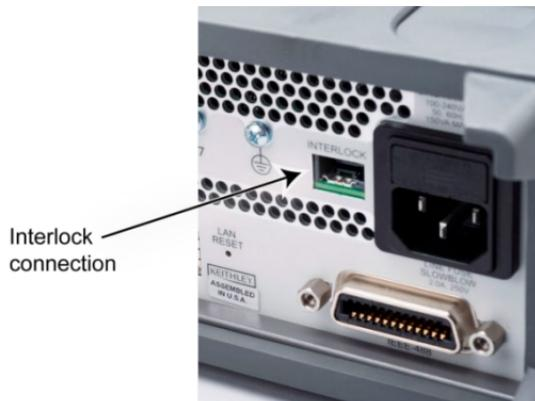
The interlock is intended for use through a normally open switch, which may be installed on the lid of a test fixture, on the enclosure of a semiconductor prober or device handler, or on the door or doors of a test equipment rack. The circuit opens when an access door is opened, and closes when the door is closed.
