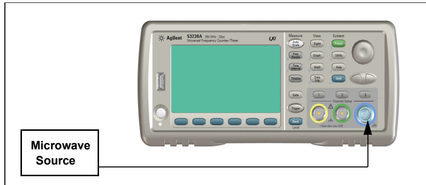
Figure 2-7. Microwave Source Connection to Channel 3
